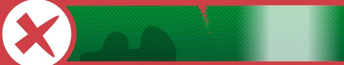
Cuts, tears, water, rock salt and oil contamination can lead to straps wearing out.
